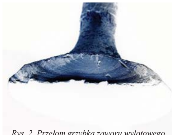
Fig. 2. Broken exhaust valve – MB820 engine
